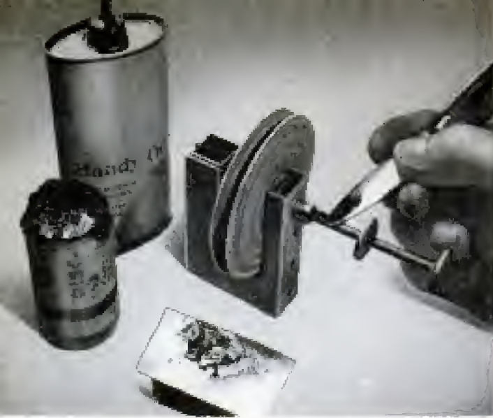
Screws often become loose and will no longer hold fine adjustment. Apply cement diluted with light oil
